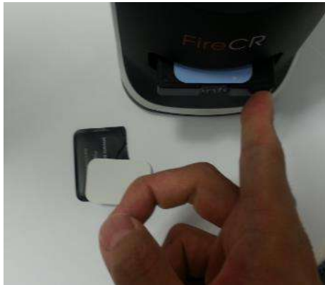
Figure 12. Push left side or right side of tray gently to start scan.
