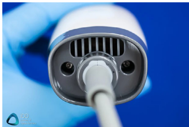
The fan vents at the back of the Helios 600.
