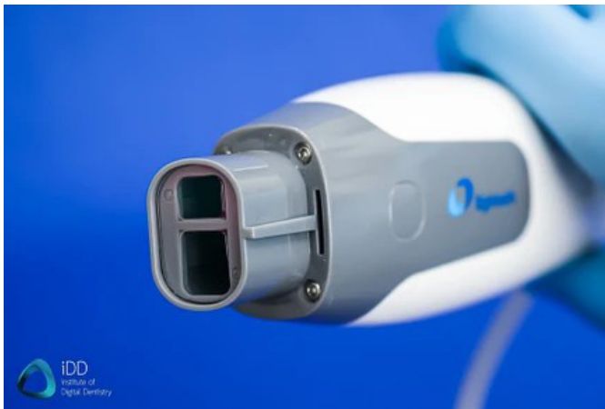
Helios 600 has non-reversible scanning tips.
