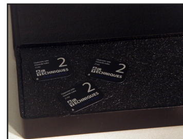
View C PSPs ready for Scanning
